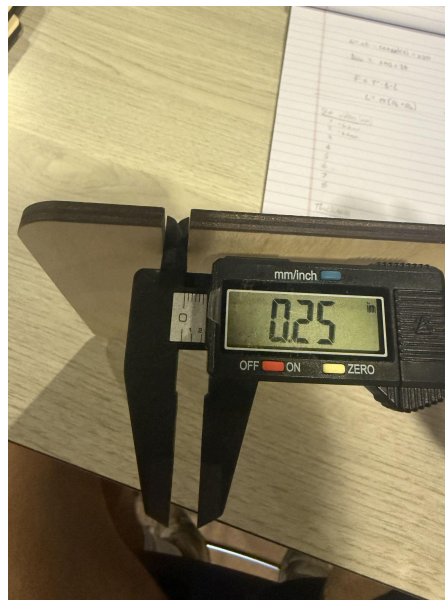
Figure 4.4: Measuring the length of the slot
