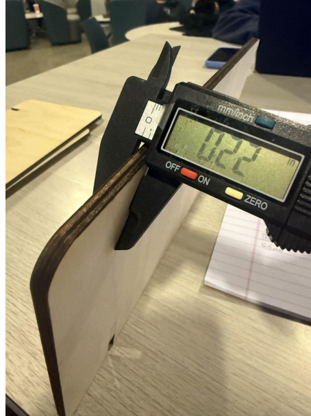
Figure 4.3: Measuring the thickness of the material
